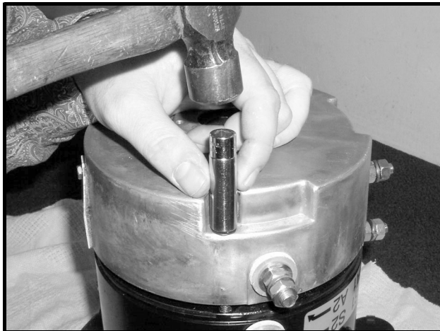
Figure 27-6 End Cap Disengagement
