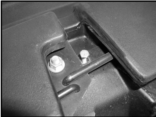
Figure 4-6 Bed Latch Link Bolt
