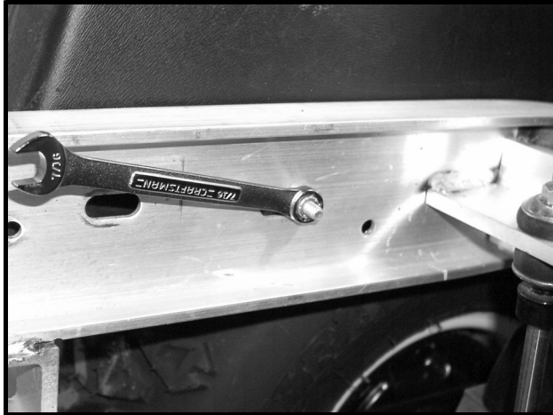
Figure 4-17 Rear Fender Frame Bolts
