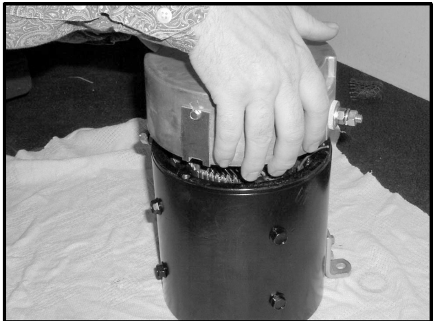
Figure 27-7 End Cap Removal
