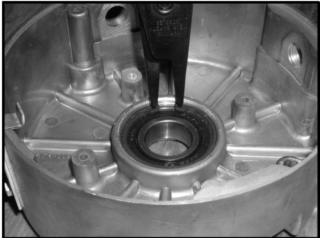
Figure 27-11 Bearing Retaining Ring
