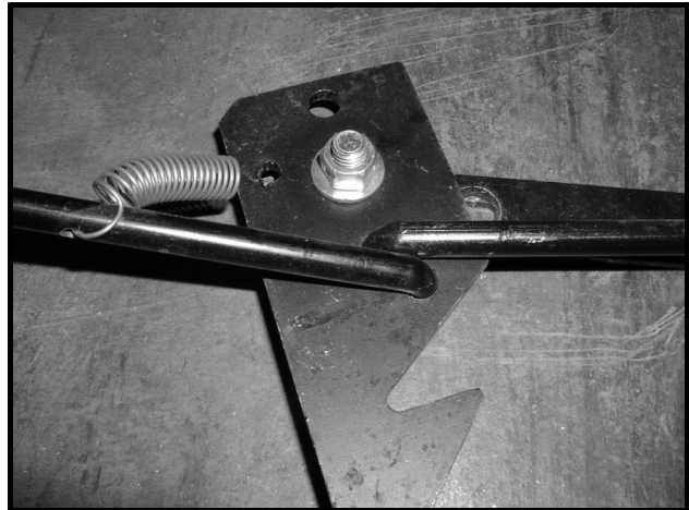
Figure 4-7 Passenger Side Catch Rods and Catch Plate
